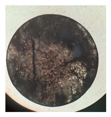
The central portion of the sample is partially transparent. However, further polishing is required to reduce the sample thickness to approximately 150 µm and determine if this improves transparency.
